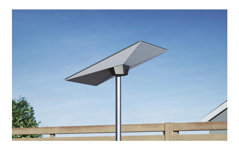
The Ridgeline Mount requires no drilling and is designed to sit on the top ridge of a gable roof. Held in place by ballast weights, the mount is ideal when you are unable or unwilling to drill holes in a roof. The mount works great with metal and shingled roofs with slopes less than 45 degrees, but is not recommended for clay tile roofs.
