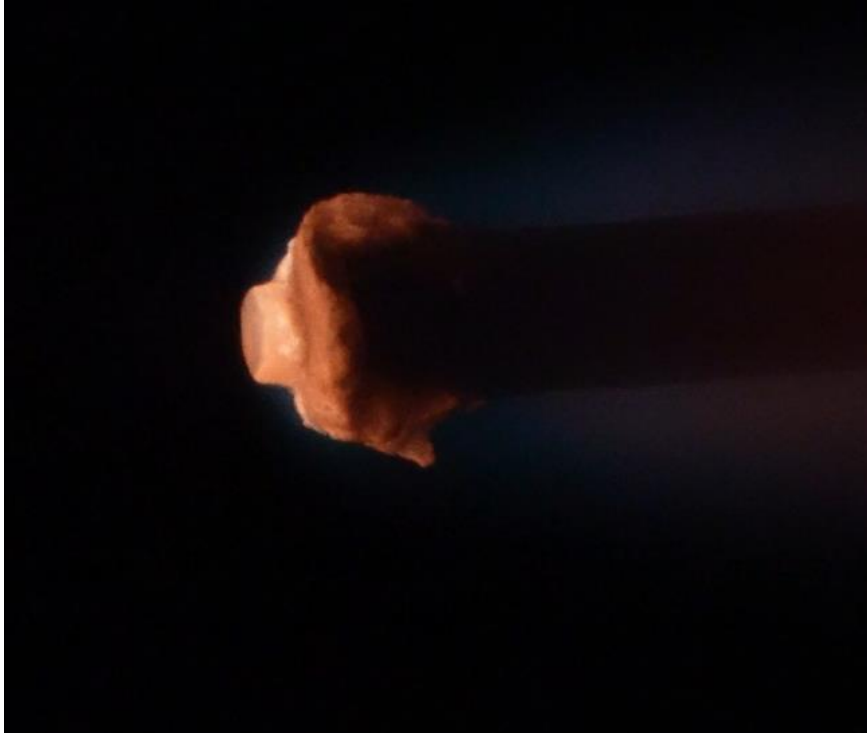
PCB at the completion of a reentry-like heating test
